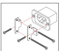
Figure 2-2. Retention Bracket Assembly
